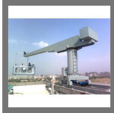
Building Maintenance Unit
